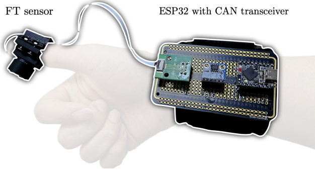
Fig. 2: Real force-data collection using a wearable F/T sensor. Contact interactions at multiple finger locations are synchronized with proprioceptive measurements.
